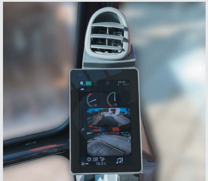
Low-reflective color 8" monitor, up to a 42% larger display compared to ZX-5G series. Easier to view and navigate. Bluetooth® and USB power supply available.
