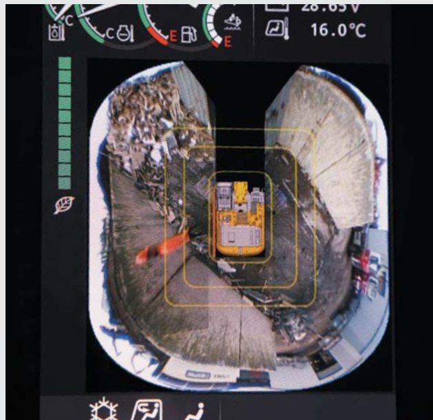
AERIAL ANGLE (Optional) 270° bird's eye-view camera system is available as an option.
