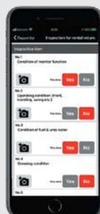
Acceptance or delivery inspection of rental machines
