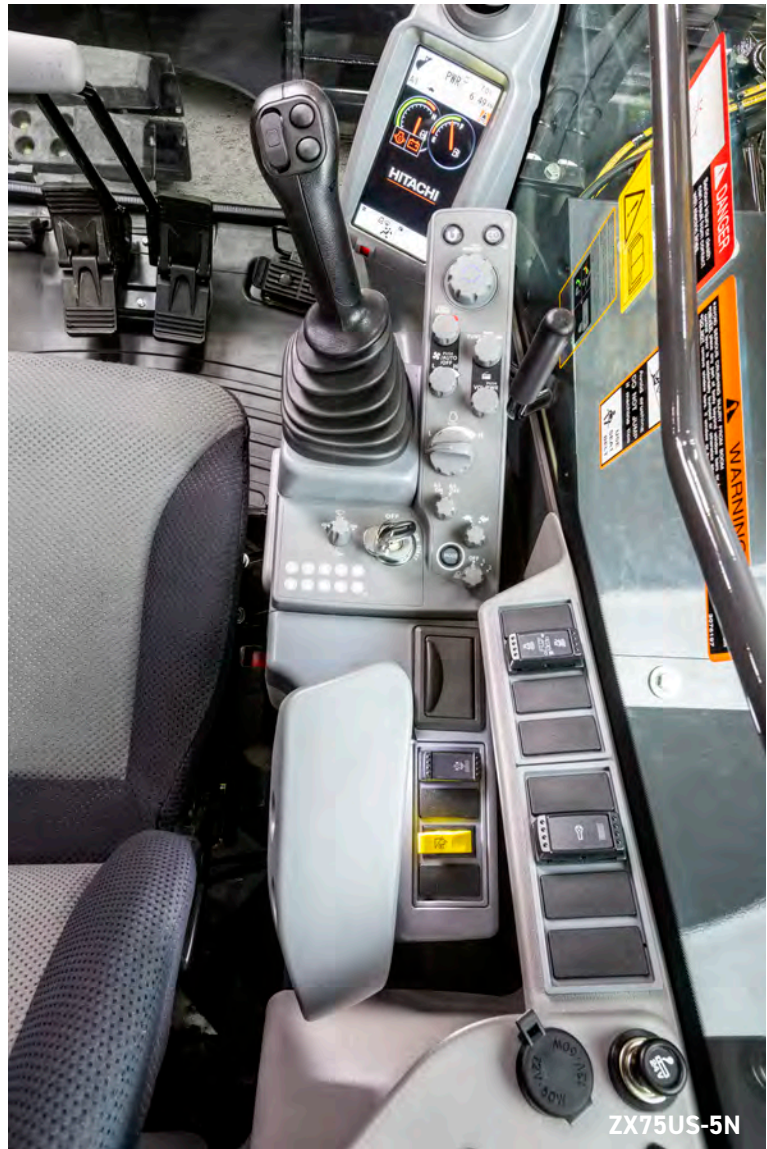
Above: Joystick controls for effortless operation and multi-function color LCD display makes operation easier.
